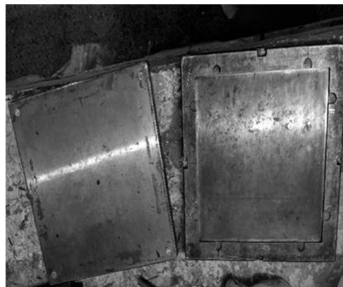
Fig 5: Mould – stain less steel (200×200×3) mm 3
