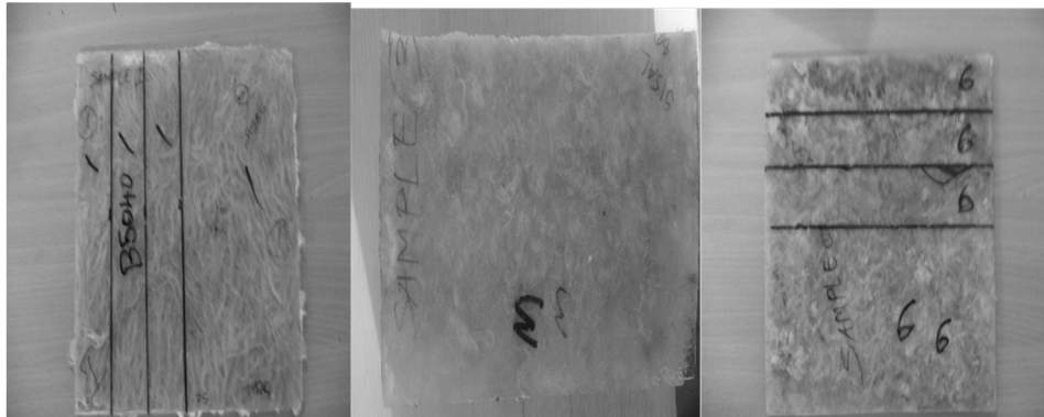
Fig 7: Prepared sisal epoxy composite for 85%-15%,80%-20% and 70%-30%
