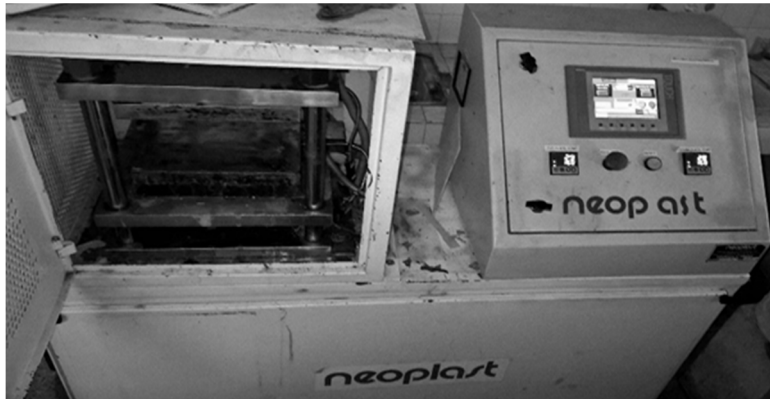
Fig 4: Neoplast compression moulding machine at CBPST, Cochin
